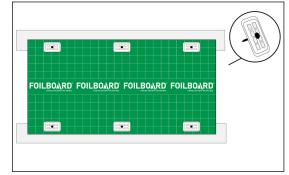
STEP 2 Fasten the Foilboard panel to the purlins using Foilboard fasteners. Use 5 or 6 per square metre.
