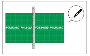
STEP 4 When cutting, measure the required area, then cut the Foilboard panel to size using a straight edge and a sharp knife.
