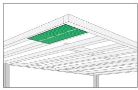
STEP 1 Position full sized Foilboard panel against the underside of the roof purlins with the anti-glare side facing out.
