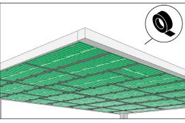
STEP 5 Tape any joins, exposed edges or gaps using Foilboard joining tape.
